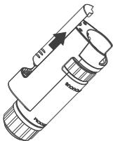
2. Install a AAA battery in the correct polarity.
