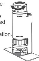
iv. Rotate the focusing ring ⑤ until the image is sharp and clear.
