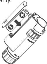
3. Attach and tighten the battery door ② as shown below.
